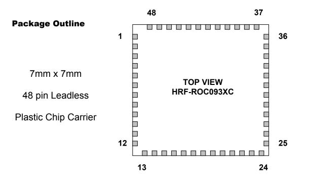
Low inductance RF/DC ground connection required below part as bottom ground pad is used for all device grounding. Additionally, this connection prodvides a direct connection to the die for enhanced thermal dissipation. *Package shown not to scale*.
